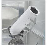
The holders are especially useful in course of weighing oval-shaped objects (bulbs, measuring vessels, test tubes etc.)
