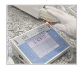
Proximity sensors stand for various ergonomic solutions, they facilitate remote control of functions such as tarring, zeroing, printout.
