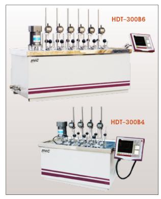
Control mode: Touch screen or PC Multi temp. measurement points Accuracy: Ternperature control range: room ternp. ~300°C 4/6 (optional). Numbers of test station:
