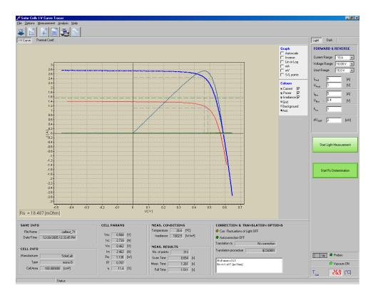
Figure 9: Example of cell's series resistance determination according to IEC 60891 & ASTM E948-09
