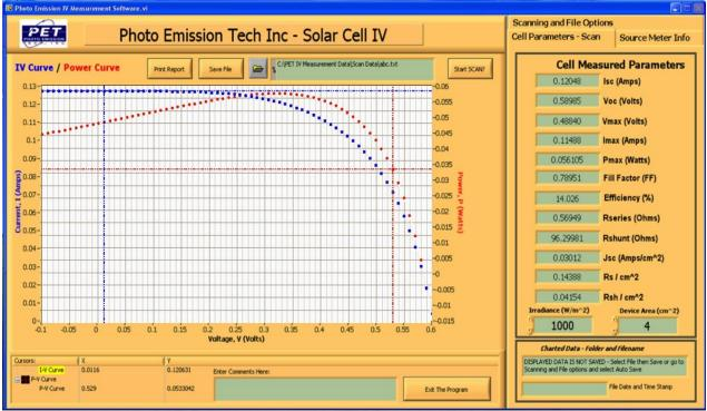
Figure 4: Cell Parameter Scan Screen
