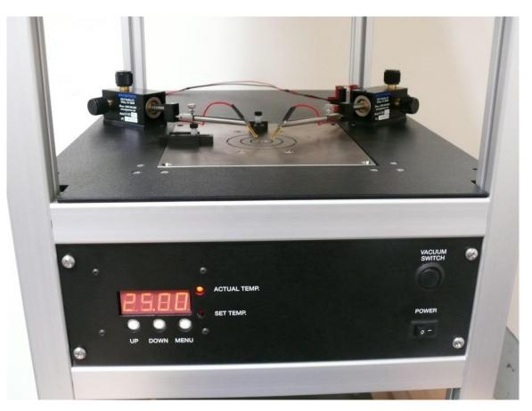
Figure 1: View of a typical cell measuring table with bottom current & voltage contacts and two (2) micro-manipulators for top cell contacts. Each Micro-Manipulator has one current & one voltage contact
