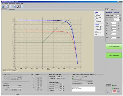
Figure 9: Example of cell's series resistance determination according to IEC 60891 Standard
