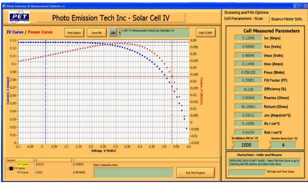
Figure 4: Cell Parameter Scan Screen
