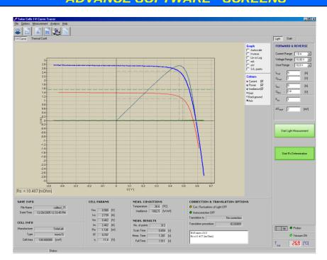
Figure 9: Example of cell's series resistance determination according to IEC 60891 & ASTM E948-09
