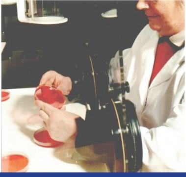
A large transfer port is fitted to the units which holds 100 Petri dishes. This port is automatically pressure pulse flushed and is fitted with a catalyst. The doors of the port are automatically sealed, locked and programmed to prevent loss of anaerobiosis. We also offer the option of an additional ten-plate entry system, in order that a small number of Petri dishes can be passed quickly into the incubator with a minimal gas usage.
