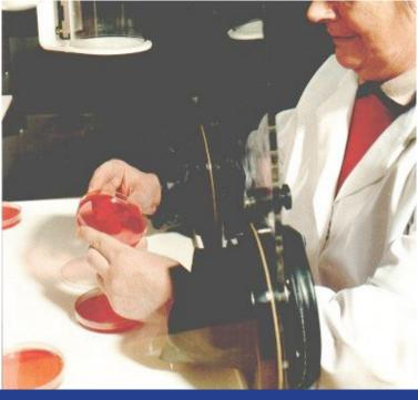
A large transfer port is fitted to the units which holds 60 Petri dishes. The outer door is hinged to reduce the overall length and the inner door slides to maximize the incubation capacity. Both doors are fitted with wear compensating seals. The units are also fitted with a single-plate entry system, situated between the arm ports at the front of the incubator. Individual Petri dishes can be passed quickly into the incubator with minimal gas usage.
