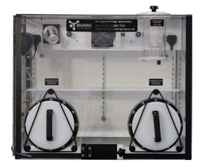
The AW300SG anaerobic workstation is ideal for the laboratory where oxygen free conditions are required for the growth and identification of bacteria. Its small bench size yet large incubation capacity makes it perfect for the individual research project. The unit is very economical to operate and works from a single cylinder of anaerobic mixed gas. The cabinet will incubate 300 Petri dishes and comes complete with catalyst sachets and plate holders.
