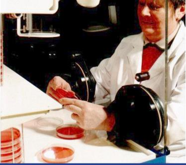
**Glove Free Operation:** This unique bare hand method is very simple to operate. Air-tight seals fit around the user's wrists as shown and the anaerobic atmosphere is maintained. The design eliminates the use of footswitches and gets rid of large internal arm port bungs, giving more working room inside the incubator. The system is very economic on gas usage and the hands can be inserted in seconds.
